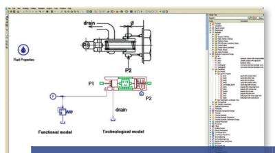
Figure 3: A simple relief valve model side-by-side with one that captures all the relevant physics to synthesize the right valve.
