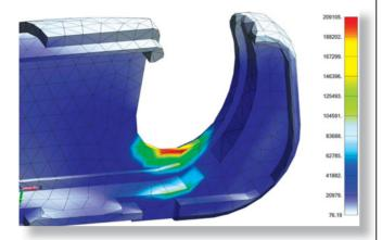
FIGURE 4: Sometimes, results seem to make no sense but are good enough if interpreted correctly. This surgical anvil has a yield strength of around 100,000 psi. With a calculated stress of more than 200,000 psi, the part has already broken. This shows the power of visualization knowledge—you know when "good enough is good enough," and remeshing would be just a waste of time.
