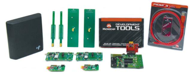
Powercast's Lifetime Power Energy Harvesting Development Kit for Wireless Sensors, created with development support from Microchip, enables wireless, RF-based battery-free operation of sensor nodes (each detects temperature, humidity and light, and an additional parameter via an external port) at a distance of 40 to 45 ft.
