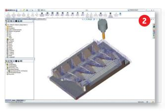
introduced an optional electrode design solution called ElectrodeWorks. It automates the calculation and design of EDM electrodes. Feature Recognition, which is used to automatically identify areas to be machined, has been upgraded to find more features while decreasing computation times by more than 50% over previous CAMWorks versions, according to the company.
