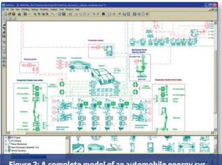
Figure 2: A complete model of an automobile energy system showing multiple libraries (differentiated by color.)
